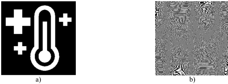
Fig. 7. The secret image is shown in part (a); the cover image with the embedded secret according to the 12-th Eigen-mode is shown in part (b).
