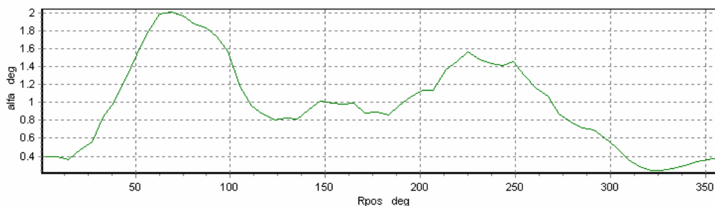
Figure 3-14 Binned standard deviation of the angle of attack associated with a low ambient turbulence situation. From [2].
