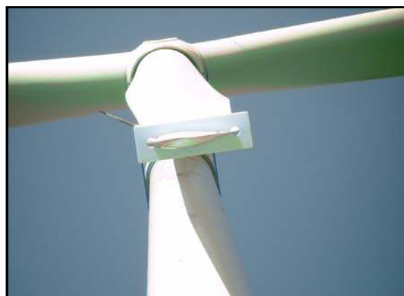
Figure 3-11 The five hole pitot tube mounted on the leading edge of the blade. (The plate mounted on the blade is used for measurement of the angle of the pitot tube relative to the tip pitch).
