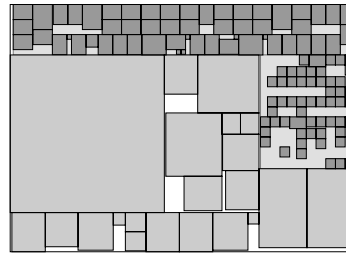
Fig. 3. A slicing floorplan obtained by using dynamic weighting Monte Carlo for a wireless modem
