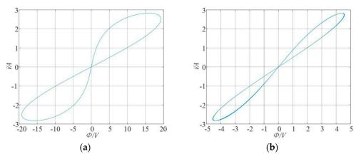
**Figure 2.** Characteristic curve of the smooth meminductor. (a) a = 1, b = 1, f = 10 Hz, (b) a = 1, b = 1, f = 50 Hz.
