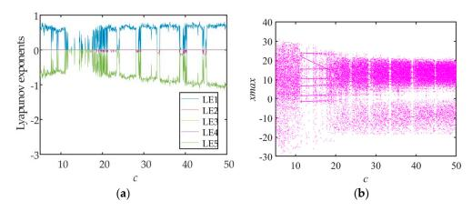
**Figure 7.** Lyapunov exponent spectrum and bifurcation diagram with parameter *c*, (**a**) Lyapunov exponent spectrum, (**b**) bifurcation diagram.
