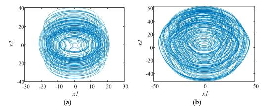
**Figure 17.** The phase diagram of attractor of DSP: (a) a = 2, b = 11, e = 1; (b) a = 0.3, b = 11, e = 7.
