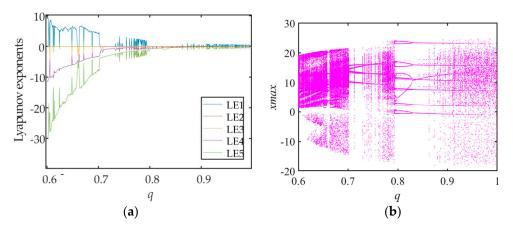
**Figure 9.** Lyapunov exponent spectrum and bifurcation diagram with order *q*, (**a**) Lyapunov exponent spectrum, (**b**) bifurcation diagram.
