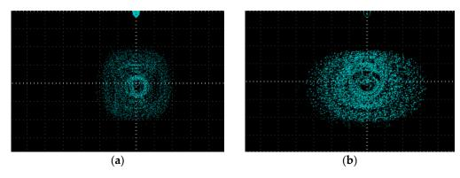
**Figure 16.** The phase diagram of attractor of DSP, (a) a = 2, b = 11, e = 1; (b) a = 0.3, b = 11, e = 7.
