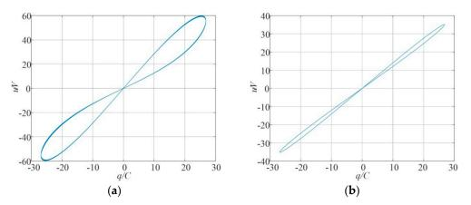
**Figure 1.** Characteristic curve of the smooth memcapacitor. (a) d = 1, c = 2, f = 20 Hz, (b) d = 1, c = 2, f = 50 Hz.
