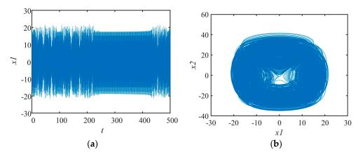
**Figure 10.** Timing diagram of the chaotic system with t = (0, 500), (**a**) time series diagram, (**b**) phase diagram of chaotic attractor.
