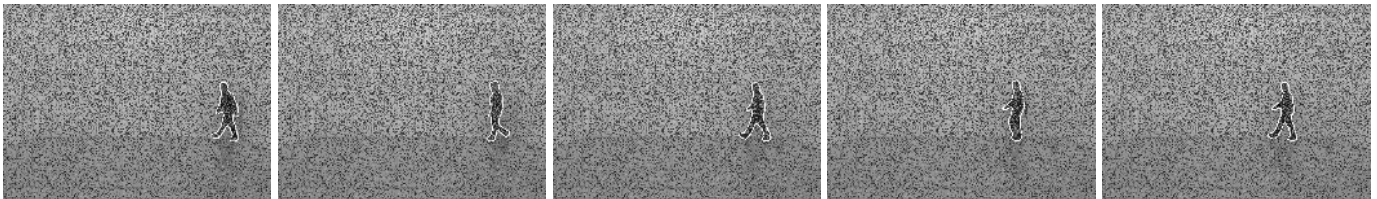
Fig. 9. Dynamical shape prior at 50% noise: In contrast to the segmentation with a static prior shown in Figure 8, the dynamical prior (using a second-order autoregressive model) imposes statistically learned information about the temporal dynamics of the shape evolution to cope with missing or misleading low-level information.
