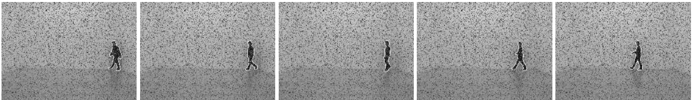
Fig. 7. Static shape prior at 25% noise: Constraining the level set evolution to a low-dimensional subspace allows to cope with some noise.
