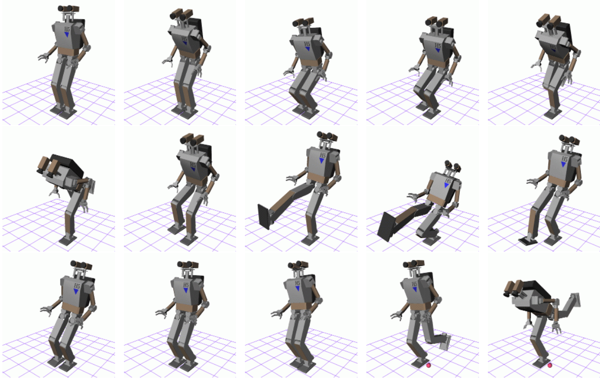
Fig. 4. Dual-leg and single-leg stable postures for the H5 humanoid robot (perspective view).
