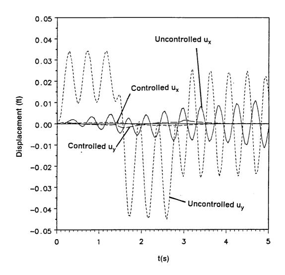
Figure 12. Tip Displacement of Beam 1
