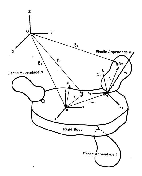
Figure 1. The Rigid Platform with Flexible Appendages
