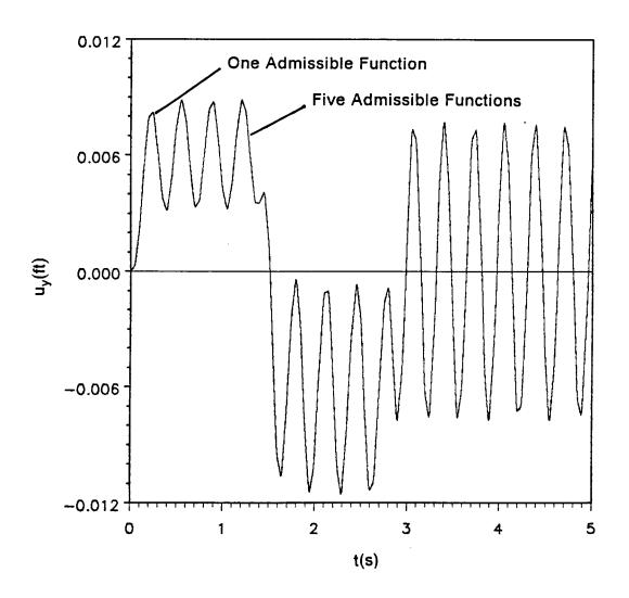
Figure 5. Time History of the Uncontrolled Tip Elastic Displacement
