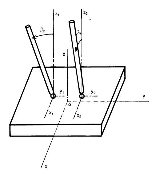
Figure 9. Rigid Platform with Two Flexible Beams
