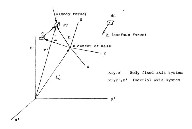
Figure 1. - Definition of axis systems used to describe the aircraft deformation.
