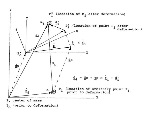
Figure 2. - Vector Diagram illustrating relationship of  $\underline{d}_i$  to  $\underline{d}_i^!$
