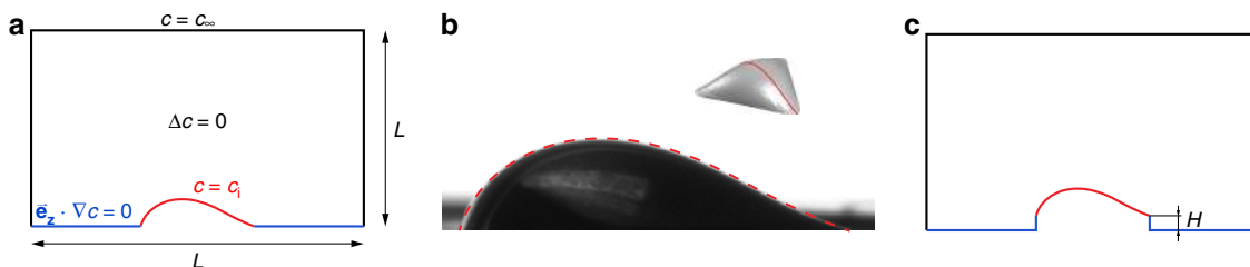
Figure 6 | 3D numerical problem. (a) Two-dimensional schematic. (b) Comparison of the experimental drop shape and the geometry calculated with Surface Evolver. (c) Problem investigating the effect of the pedestal height. Note that the schematics are not to scale and the simulations are in 3D.
