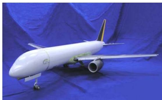
Figure 20. Photo of Generic Transport Model sub-scale flying testbed.
