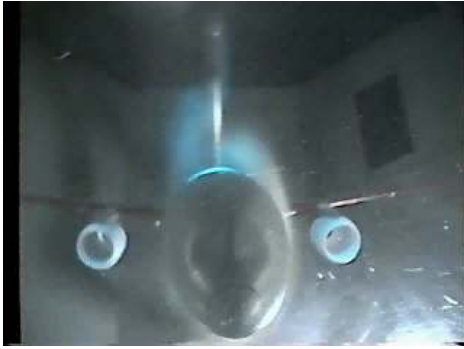
Figure 12. Photo of flow visualization results showing unsteady flow field at \alpha=60^\circ .
