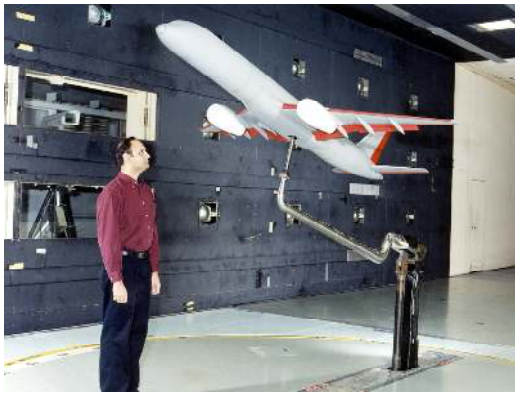
Figure 4. Photo of 5.5% sub-scale wind tunnel model in the LaRC 14- by 22-Ft Tunnel.
