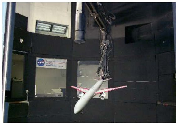
Figure 5. Photo of 3.5% sub-scale wind tunnel model in the LaRC 20-Ft Vertical Spin Tunnel.
