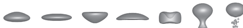
Figure 8 | A new breakup mode in region IV for Ga=500 and Eo=1 . Bubble shapes are shown at dimensionless times (from left to right) t=2, 4, 6, 7, 8, 9 and 9.1 .
