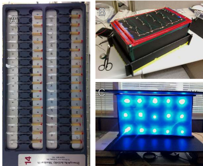
Figure 3.1: Equipment for Drosophila behavior experiments. (A) Drosophila Activity Monitor (DAM). Cuvettes containing individual flies with food are placed in slots in the DAM where movement is registered by the cutting of a light beam. (B) Top view of foam board box for light-resetting experiments. (C) Inside view of a partially-deconstructed box, showing light from 15 blue LEDs passed through a sheet of diffusing plastic.
