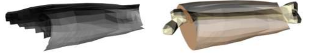
Figure 2: Modeling of a thigh finite element model using a skeleton and CSG operations.
