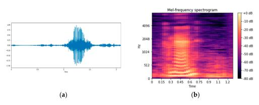
Figure 4. Feature extraction: (a) voice signal and (b) mel spectrum.
