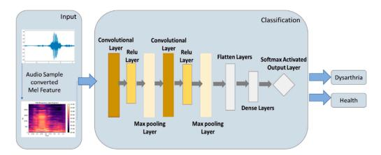
Figure 5. Architecture of CNN model.
