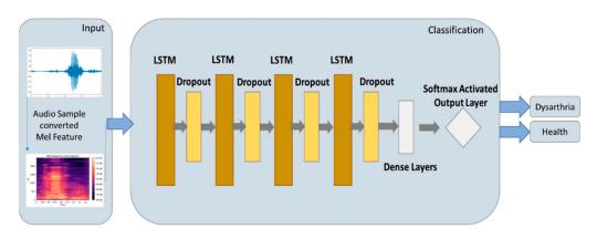
Figure 6. Architecture of LSTM model.
