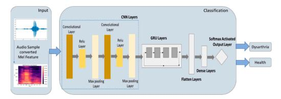
Figure 8. Architecture of CNN-GRU model.
