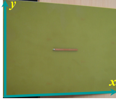
Fig. 7.a: Photograph of the tested device ( L_x \times L_y = 210 \text{ mm} \times 170 \text{ mm} ).
