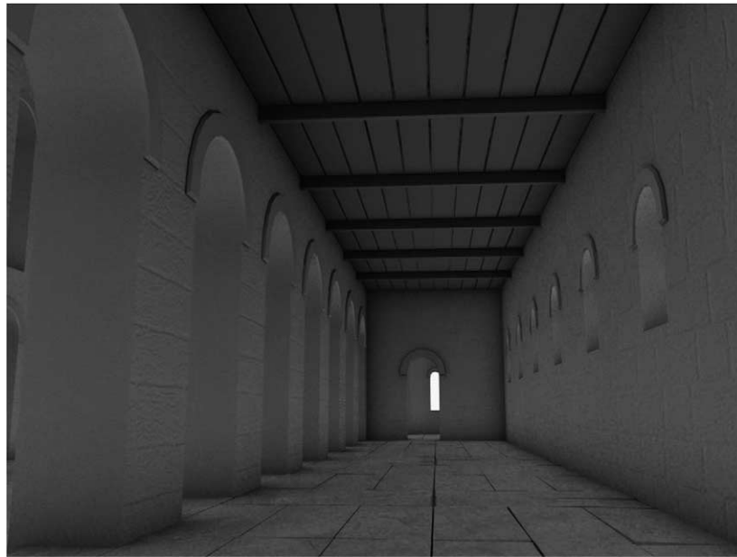
Fig. 9. Phong haptic shading rendering: A point-perspective view of the Aghios Achilleios basilica CAAD model (haptic representation based on digital low-resolution Canon CI-10 imagery).
