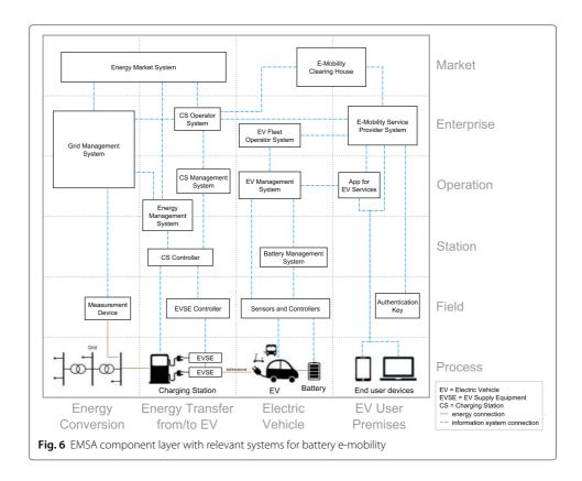
hardware/software components for battery-electric mobility are shown. The components for non-battery e-mobility are excluded for reasons of clarity and comprehensibility. To comply with the case study in the validation section, here the focus is limited to battery-electric mobility.
