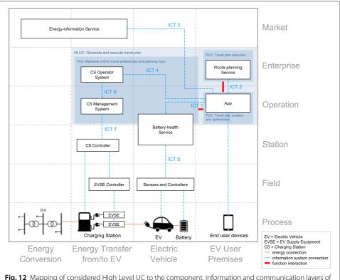
**Fig. 12** Mapping of considered High Level UC to the component, information and communication layers of EMSA Model
