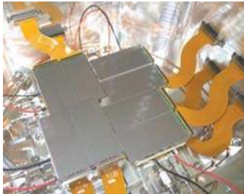
Figure 14. (a) Single sensor in test camera and (b) eight sensors in x-ray free-electron-laser camera
