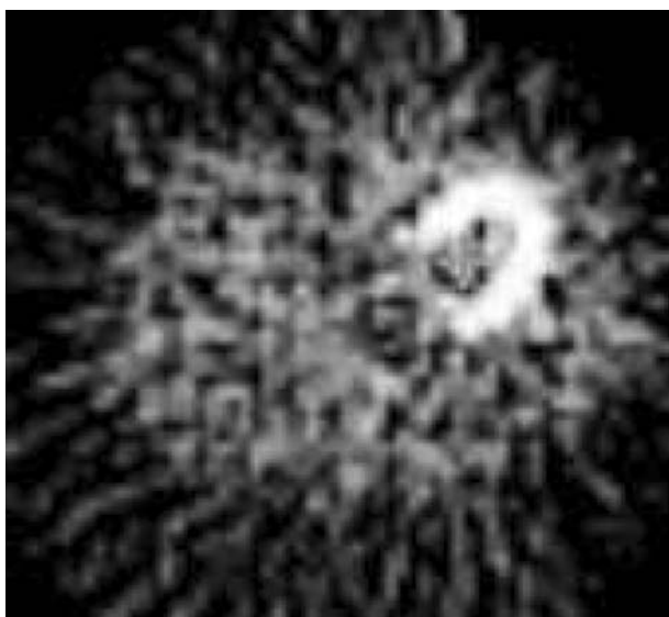
Fig. 4. Streak artefacts with FBP. Illustration of streak artefacts inherent to the FBP process
