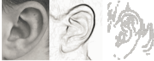
(c) Original image, edge enhanced image and corresponding edge orientation model [62]
