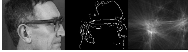
(a) Original image, edge image and Hough transform [38]
