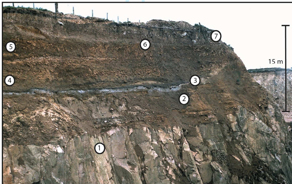
Figure 18 South Face 1 of Kirkhill Quarry in the late 1970s. 1. Floor of meltwater channel cut in a felsite dyke. 2. Pitscow Sand and Gravel Formation. 3. Kirkhill Palaeosol Bed. 4. Camphill Gelifluctate Bed. 5. Rottenhill Till. 6. Corsend Gelifluctate Bed. 7. Hythie Till.
