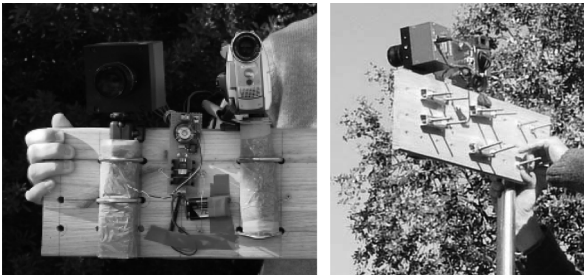
9 10 Fig. 9: Arrangement of the EyeRIS™ system (on the left in both photos) and the commercial 11 camcorder (on the right in both photos) during the field tests.
