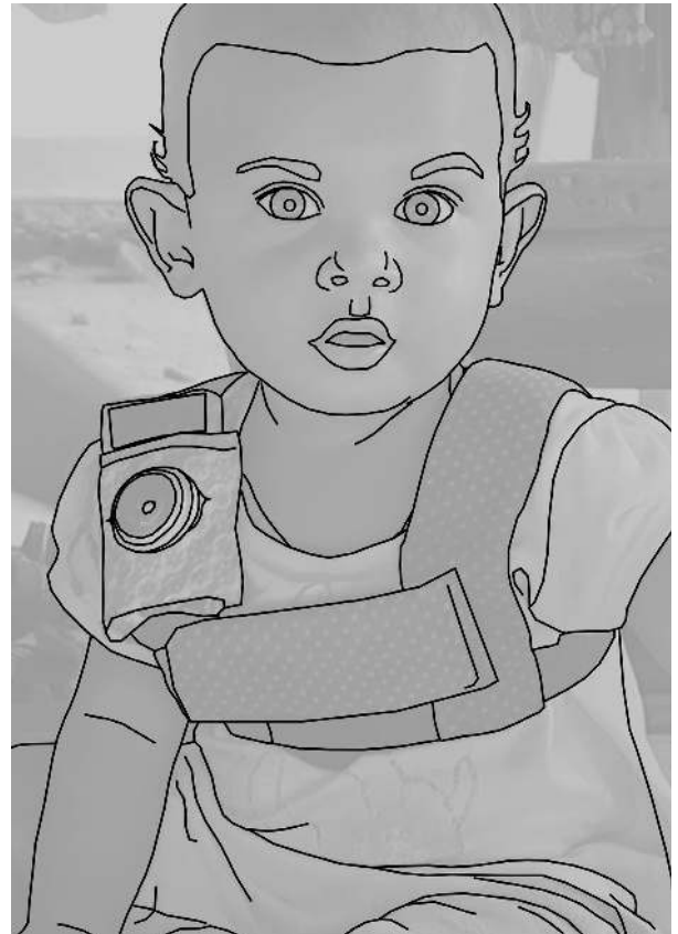
Figure 1. The recording vest included an Olympus audio recorder in the front horizontal pocket and a miniature camera with a fish-eye lens on the shoulder strap.
