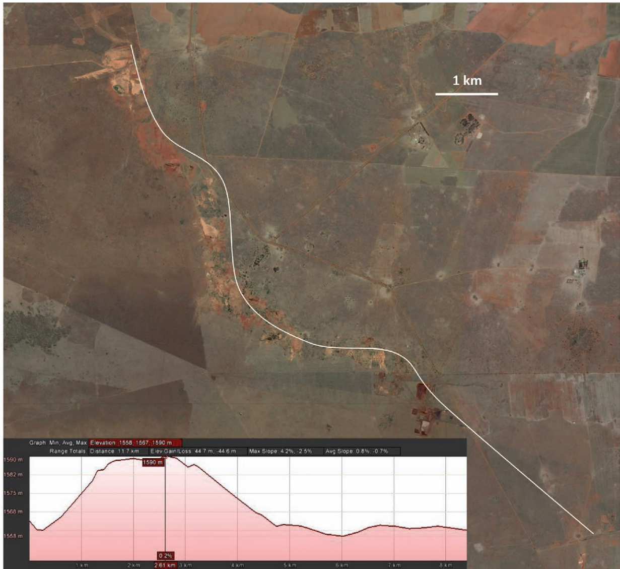
Figure 8. Profile of the Goedgedacht 'run' showing the major uphill section in the upper part of the run as well as its overall zero gradient (Google image as background).
