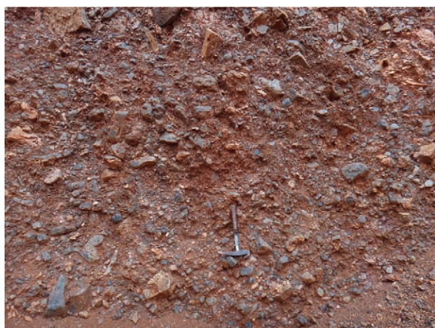
Figure 10. Clast-supported massive diamicrite (Dcm) lithofacies from the Manana run. Note the shape variations of the clasts. Hammer for scale.
