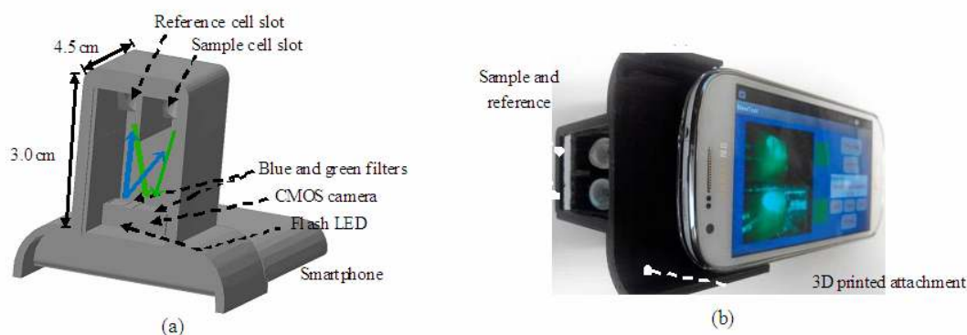
Fig. 2 Structure of the smartphone fluorimeter: (a) the smartphone attachment designed in AutoCAD Inventor Fusion, and (b) photograph of the 3D printed attachment installed on an Android-based smartphone.
