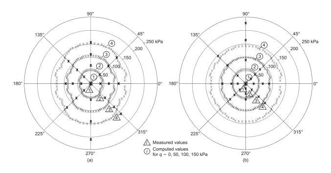
Fig. 17. Results of analysis B: (a) radial pressures on the pipe at r = 107 mm in the loose backfill; (b) radial pressures on the pipe at r = 107 mm in the compacted backfill
