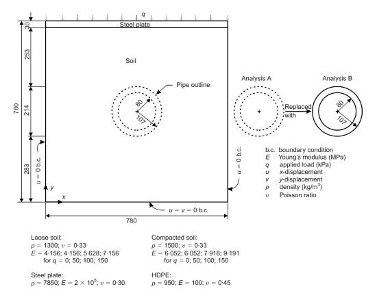
Fig. 16. FLAC model for analysis A and analysis B (all dimensions are in mm)
