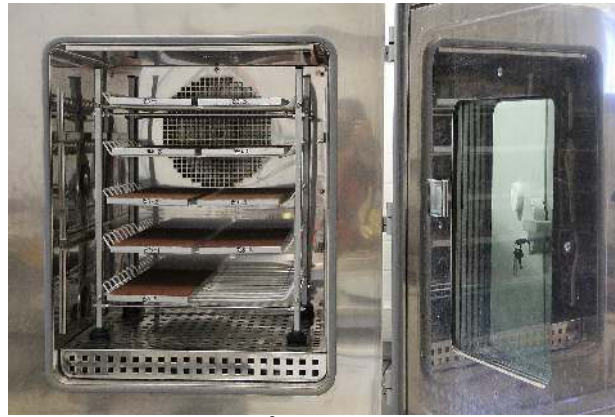
Fig. 5 – Climatic chamber with the 1000 cm 2 mortar samples for adsorption and desorption tests
