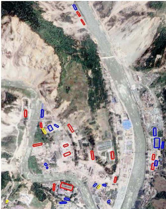
Fig. 10. Footprints of selected buildings overlaid to the post-QB image, giving an overview of the distribution of the candidates in the test set. Buildings of class \omega_d are marked with red polygons, while blue polygons correspond to the class \omega_u . The yellow polygons show the three buildings where the true status in the post-TSX and post-CSK is unknown. (QuickBird images: Copyright 2008, DigitalGlobe distributed by Eurimage S.p.A.)
