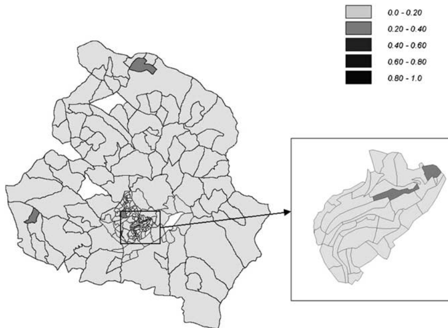
Figure 7. Map of the mean damage in each census tract of the whole Potenza territory and its historic centre (50 years return period, site effects not included).
