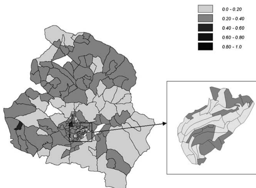
Figure 9. Map of the mean damage in each census tract of the whole Potenza territory and its historic centre (50 years return period, site effects included).
