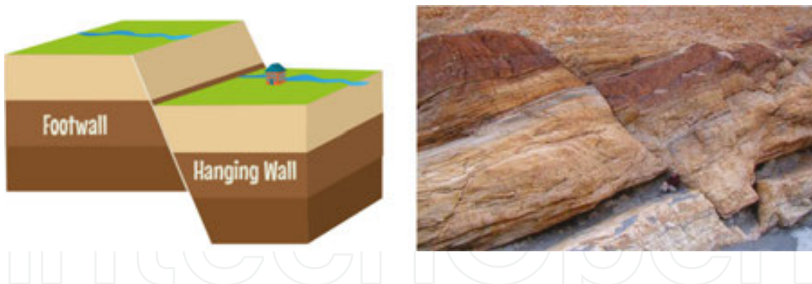
Figure 5. Normal fault graphical presentation and mechanism [7].
