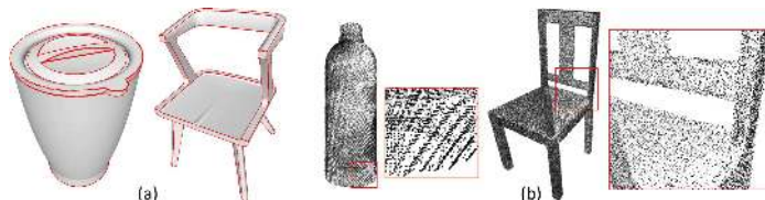
Fig. 3: Example annotated edges (in red) on some of our collected 3D meshes (a). Example point clouds produced from our virtual 3D scans (b). The point density varies and the zoom-in windows also reveal the synthetic noise.
