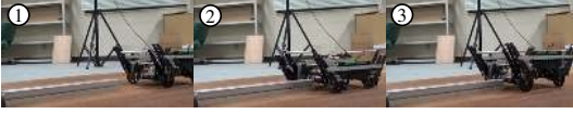
Fig. 20. Protrusion traversing experiment with crank model. This model could not successfully traverse the protrusion because its clearance height was lower than the protrusion; consequently, the body interfered with the protrusion.
