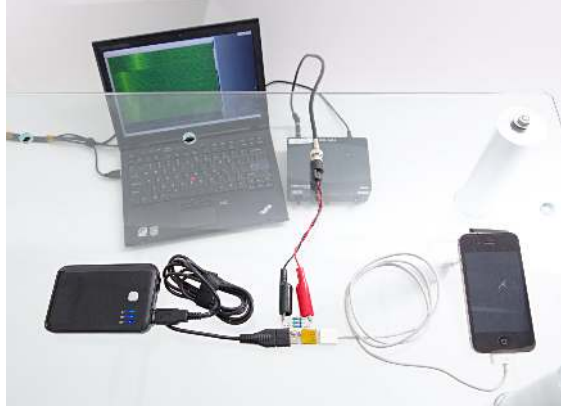
Figure 9: Mounting a cheap power analysis attack on an iPhone 4 through its charging port. This setup includes a portable battery (bottom, left), a power monitoring probe (bottom, middle) and an iPhone 4 (bottom, right). The power probe is then connected to the Tracker Pre sound card (top, middle) and the attacker’s laptop (top, left).
