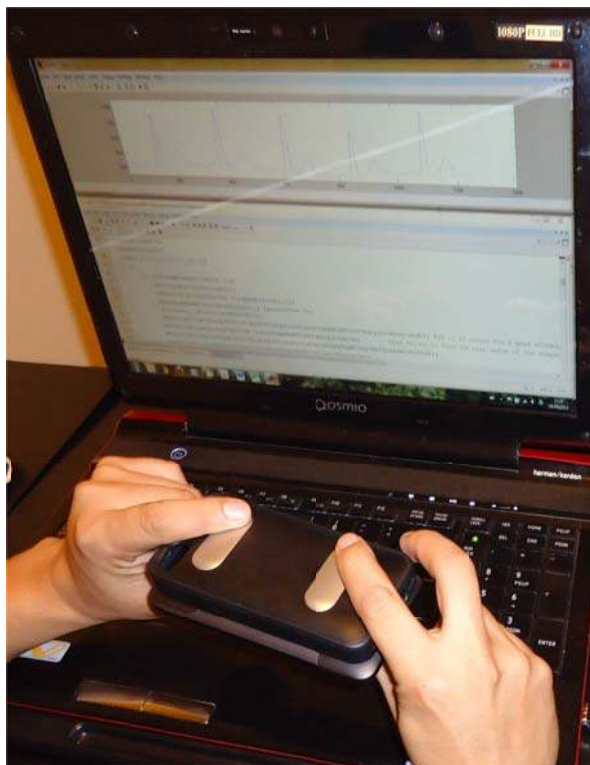
Figure 4-14: Signal acquisition for ECG mobile authentication.
