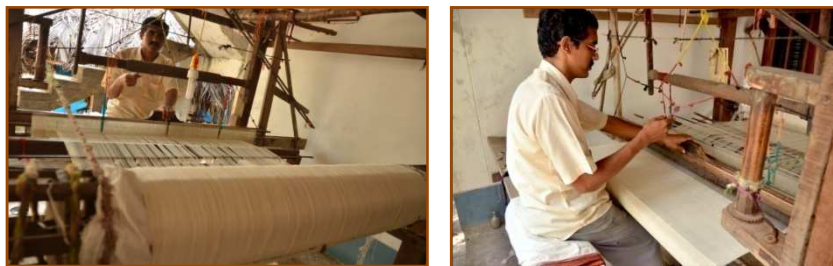
Figure 2: Weaving of Sisal Union Fabrics on Handloom
