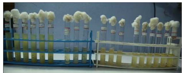
Fig. 1 MPN test at premonsoon season in S-I site of Subarnarekha river water
