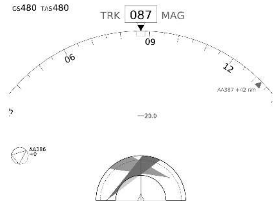
Figure 10. Display for airborne self separation showing velocity obstacles.
