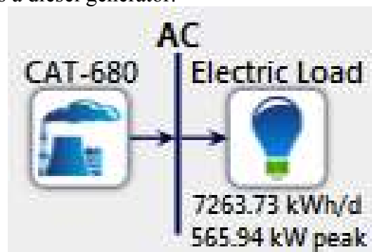
Figure 3.6: Schematic for stand-alone diesel generator in islanded mode.
