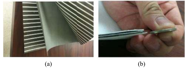
Fig. 4. The structure of textile sensor and sensor array design. (a) Sensor implementation. (b) Sensor thickness.
