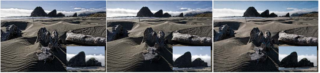
Figure 7: (left) Results by the multi-scale bilateral filter Fattal et al. [2007], (middle) Farbman et al. [2008], and (right) using the WRB edge-avoiding wavelets (with \alpha = 1 ). The mountain blow-ups show the artifacts due to gradient-reversals in the multi-scale bilateral filter.
