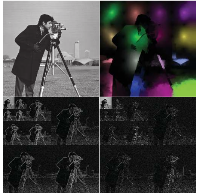
Figure 3: (top-left) Input image, (top-right) a few dual WRB scaling functions, from the third level ( j = 3 ), are shown with unique colors, (bottom-left) translation-invariant red-black wavelet transform, and (bottom-right) weighted red-black wavelet transform (computed with \alpha = 0.8 ).
