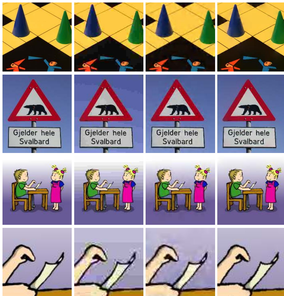
Fig. 2. Comparison of compression methods for different test images. Rows from top to bottom: coppit ( 256 \times 256 ), svalbard ( 380 \times 431 ), comic ( 512 \times 512 ), comic (detail) ( 100 \times 100 ). Columns from left to right: original image, JPEG, JPEG2000, and PDE-based compression using contours (sampling distance d from top to bottom: 5, 5, 5; quantisation parameter q : 4, 5, 5).
