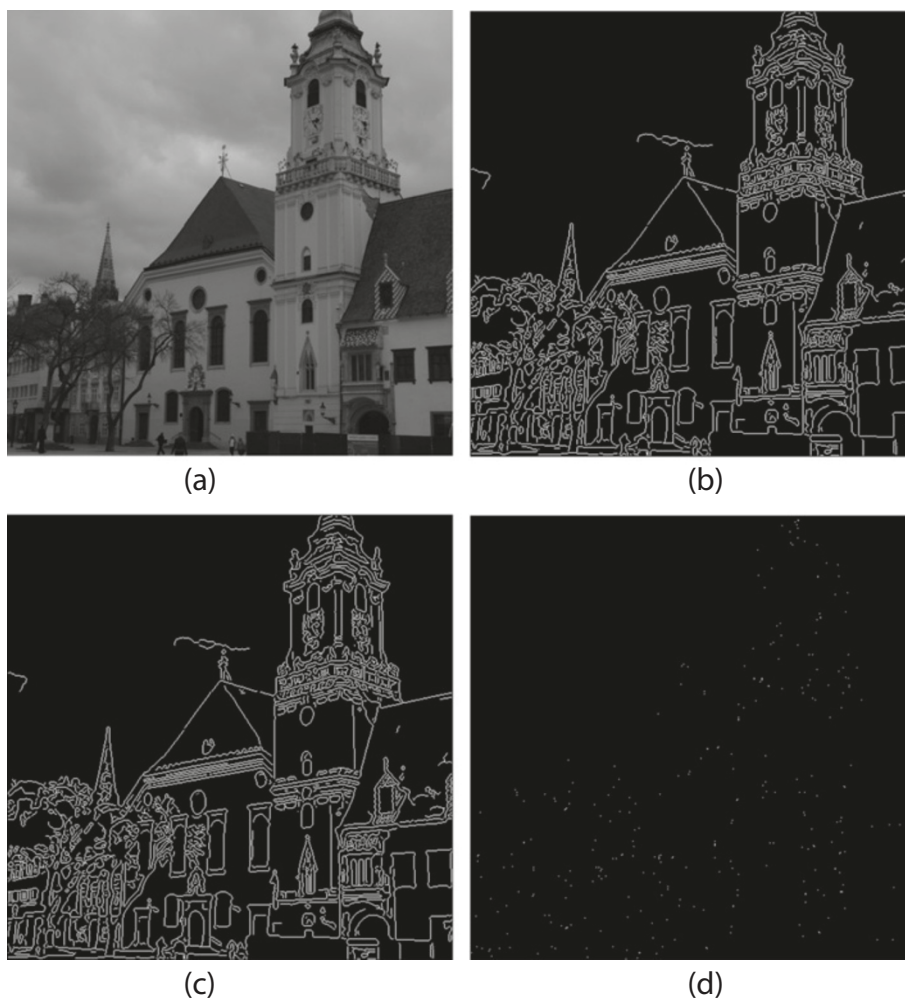
Figure 2 Change in the number of edge pixels due to embedding. (a) Cover image. (b) Edge pixels in a cover image. (c) Edge pixels in a stego image. (d) Edge pixel mismatch.
