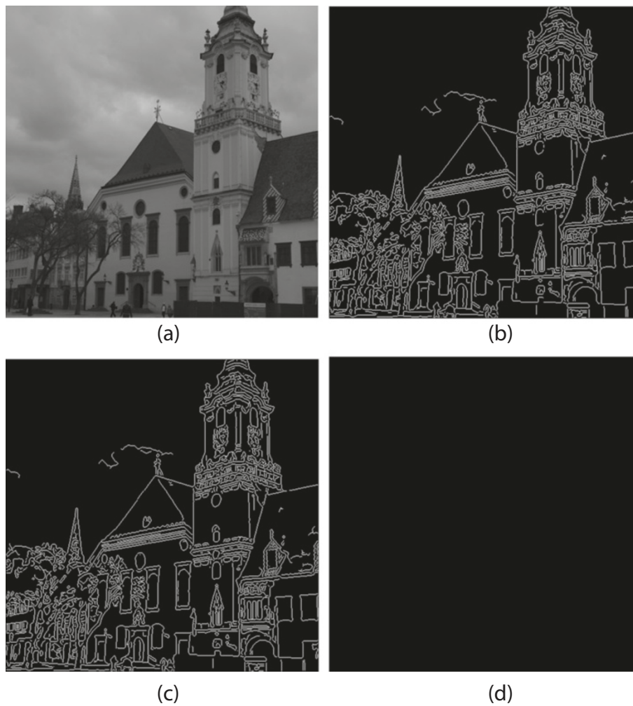
Figure 3 Change in the number of edge pixels due to embedding. (a) Cover image. (b) Edge pixels in a cover (masked). (c) Edge pixels in a stego (masked). (d) No edge pixels mismatch.
