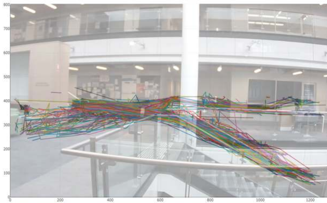
Figure 15. Trajectories followed by the individuals detected and tracked by the sensor. Each of the 631 lines represent one individual.
