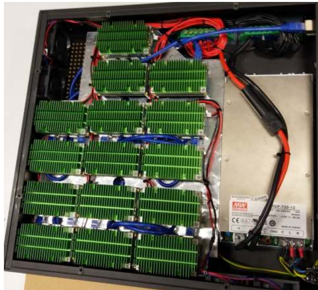
Figure 5. The 3U server version of the visual sensor hosting 15 NVIDIA Jetson TX2 units, each of these computing modules are able to process in real time one live video feed from a CCTV camera.
