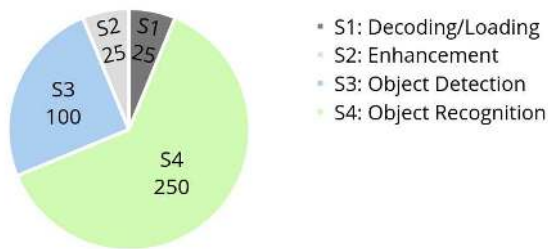
Fig. 7. Time to process stages of an object recognition job in milliseconds (ms)
