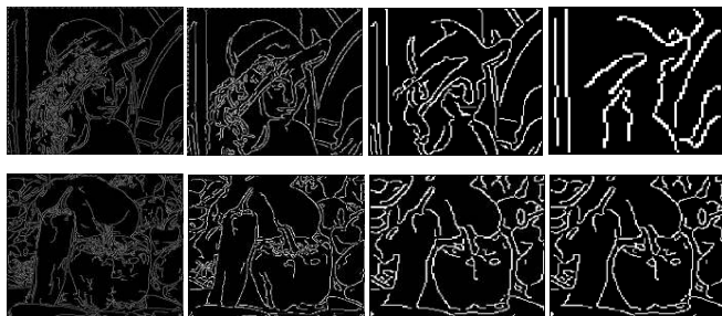
Fig. 6. Canny edge detector output for multi-scale Lena and Peppers at scales from left to right: (a) 512^2 , (b) 256^2 , (c) 128^2 , (d) 64^2 .
