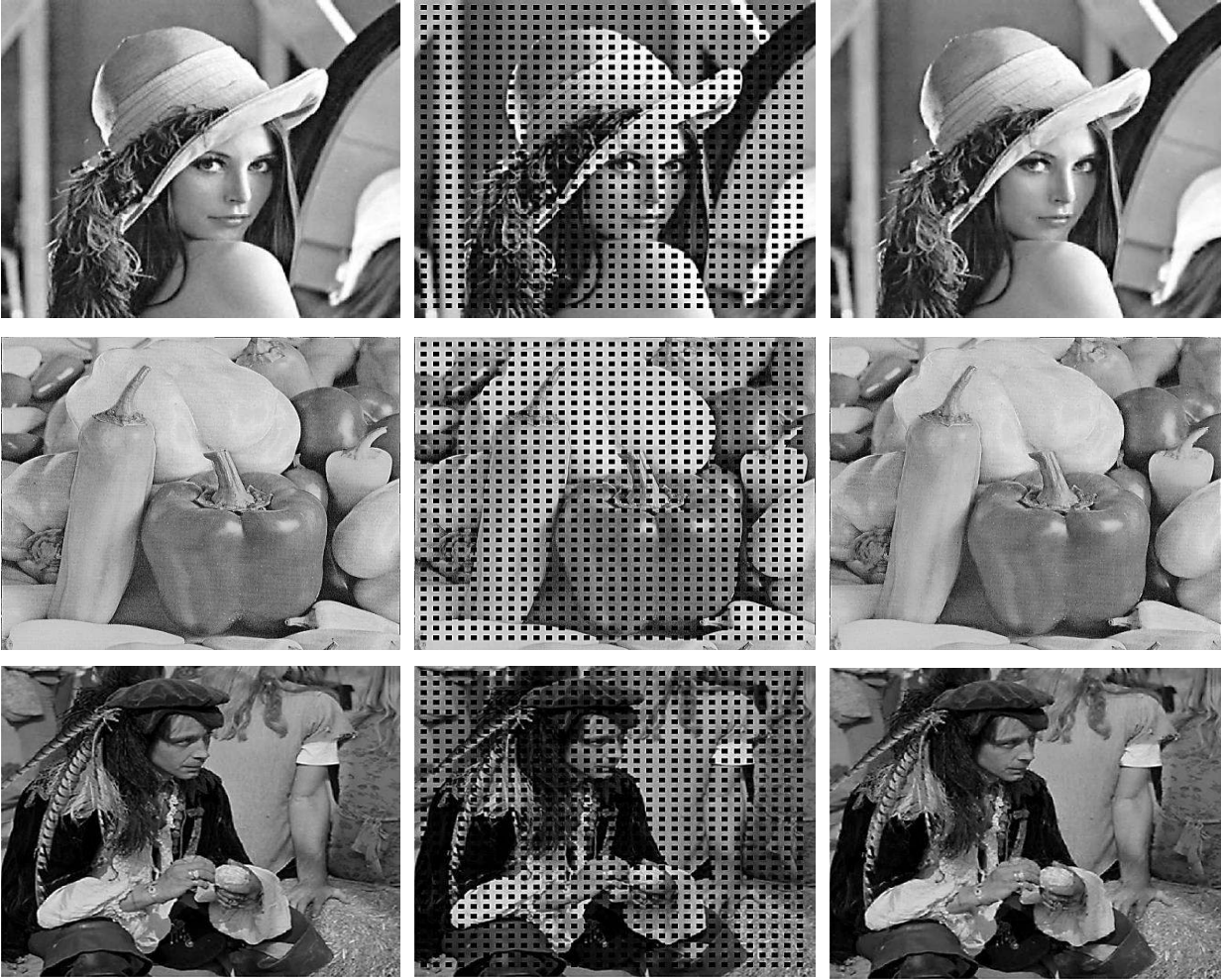
Fig. 10. From left to right; the original images, the image with 25% regular pattern loss and the restored images for Lena, Pepper and Man.
