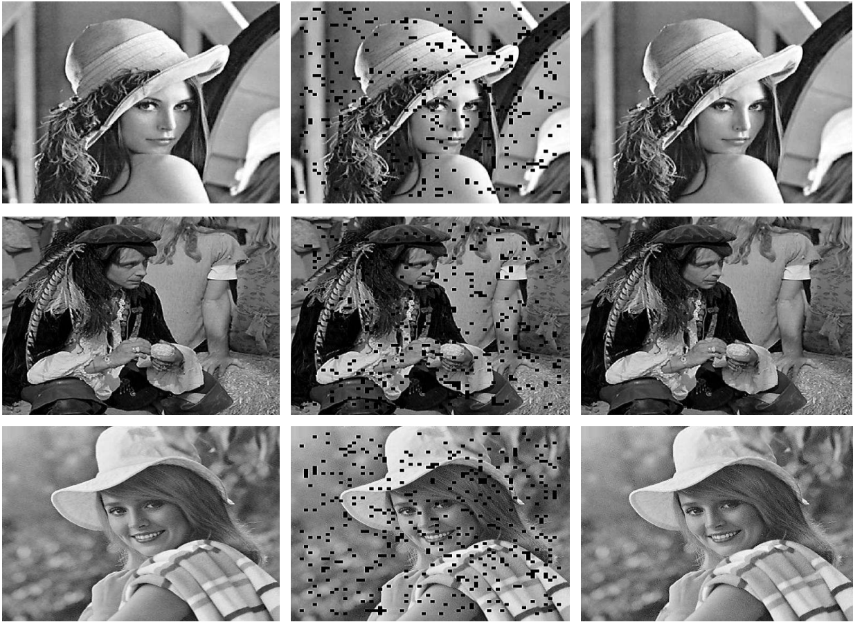
Fig. 12. From left to right; the original Lena, Man and Elaine images, the image with 10% random loss and the restored image.
