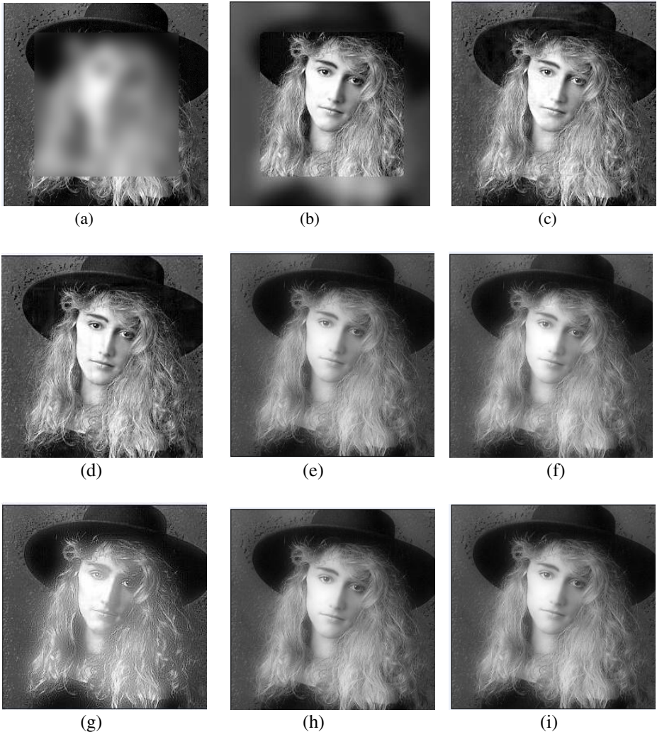
Fig. 2. Fusion results for multifocus images. (a). Source image 1, (b). Source image 2, (c). Fused image by the proposed fusion method, (d). DWT maximum fused image, (e). DWT average fused image, (f). DWT average-maximum fused image, (g). SWT maximum fused image, (h). SWT average fused image and (i). SWT average-maximum fused image.
