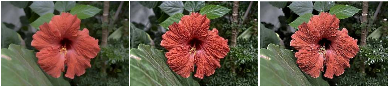
Figure 11: Fine-scale enhancement of the input image (left) using WLS [Farbman et al. 2008] (middle) and our technique (right) provides similar results with subtle differences since the detail on the petals are of, both, low contrast and fine scale. The WLS method fails to enhance fine-scale detail that are high-contrast such as the serrations on the leaves in the background and specularities on the small leaves on the right. In addition, coarser features such as the subtle discoloration on the defocused top-left portion of the image are enhanced as detail by the WLS method simply because they are low contrast.
