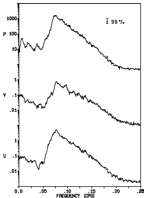
Fig. 4. Spectral estimates of pressure p ( \text{kPa}^2/\text{cps} ), Offshore velocity u ( \text{m}^2 \text{s}^{-2}/\text{cps} ) and alongshore velocity v ( \text{m}^2 \text{s}^{-2}/\text{cps} ) from the southern Seadata. Each estimate was calculated by ensemble averaging over the spectral and cross-spectral estimates for 48 consecutive bursts, giving 96 degrees of freedom.
