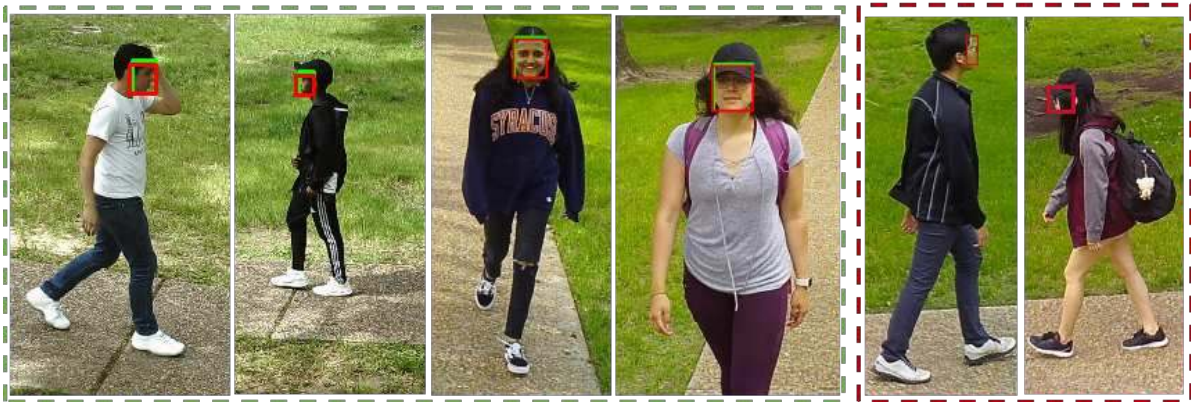
Figure 7: Qualitative results of SANet on EDGE20 dataset for the face detection problem. In each image, red boxes denote groundtruth, and green boxes denote results of SANet. Images in the dashed-green box represent success detection results, and the images in the dashed-red box represent failure cases.
