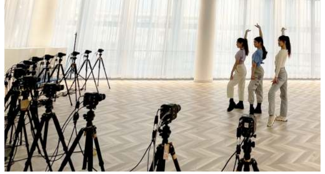
Fig. 10. Illustration of our capture system. It consists of 16 RGB cameras to cover a view range up to 180 degrees for various dynamic scenes. All the cameras are synchronized and fixed during capturing.
